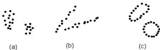
Figure 1 – Examples of data cluster types: a) cloud-type b) line-type c) circle or shell types
